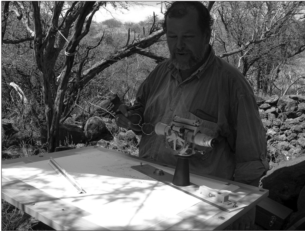
Figure 1. Pat Kirch mapping a domestic structure on the Big Island of Hawai'i in 2007. Learning the fine art of telescopic alidade and plane table mapping is a familiar rite of passage for many of Kirch's students, one which we carry on proudly when doing our own survey work.
