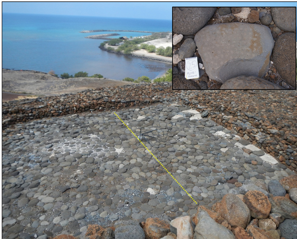
Figure 4. A portable XRF (x-ray fluorescence) mounted on a tripod in the process of non-destructively determining the geochemistry of the main paving stones of Pu‘ukoholā Heiau. Results reflect two groupings, one consistent with Pololū Series (Type I) and one with younger Hawi Series (Type II) stone (Tables 1 & 2). While these are consistent with Pololū Valley geology, which contains potential building stones from both series, without further study we cannot eliminate the possibility that these also include local stone from nearby gulches and/or stone from other locations.
