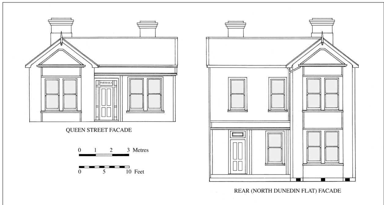
Figure 15. Reconstructions of the front and rear elevations of ‘Parihaka House’ as it probably appeared in 1880, based on examination of the house in 2015. The main uncertainties are the presence of either one or two doors that opened onto the rear veranda, and the use of a single or double sash window in the front wall.
