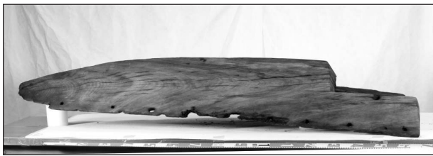
Figure 15. The Paekakariki bow piece with lashing holes around the edges for the attachment of strakes and a prow, and with a mortice and tenon joint for attachment to the main hull.
