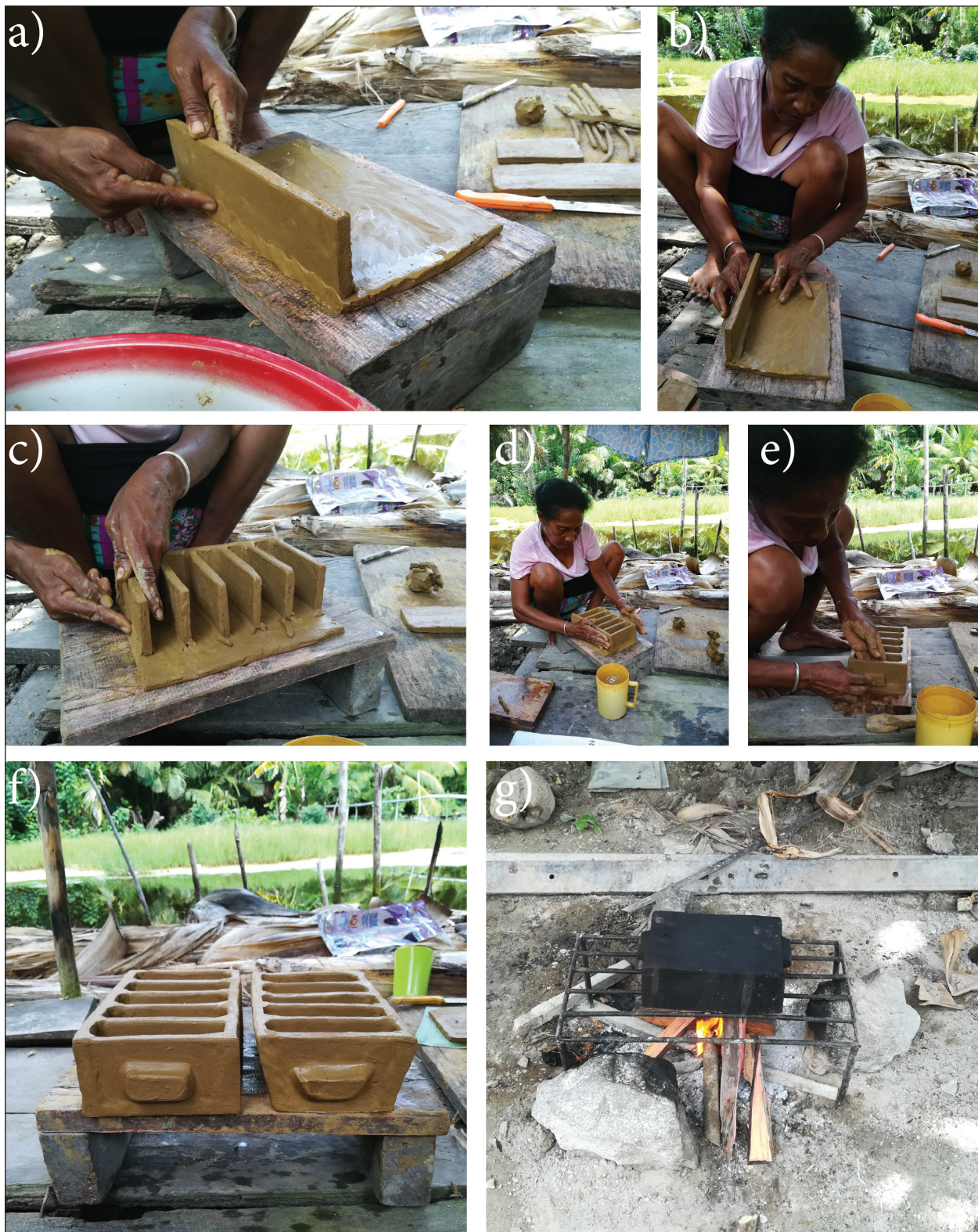
Figure 6. Assembly, drying and firing stages of sago oven production at Arefi.
