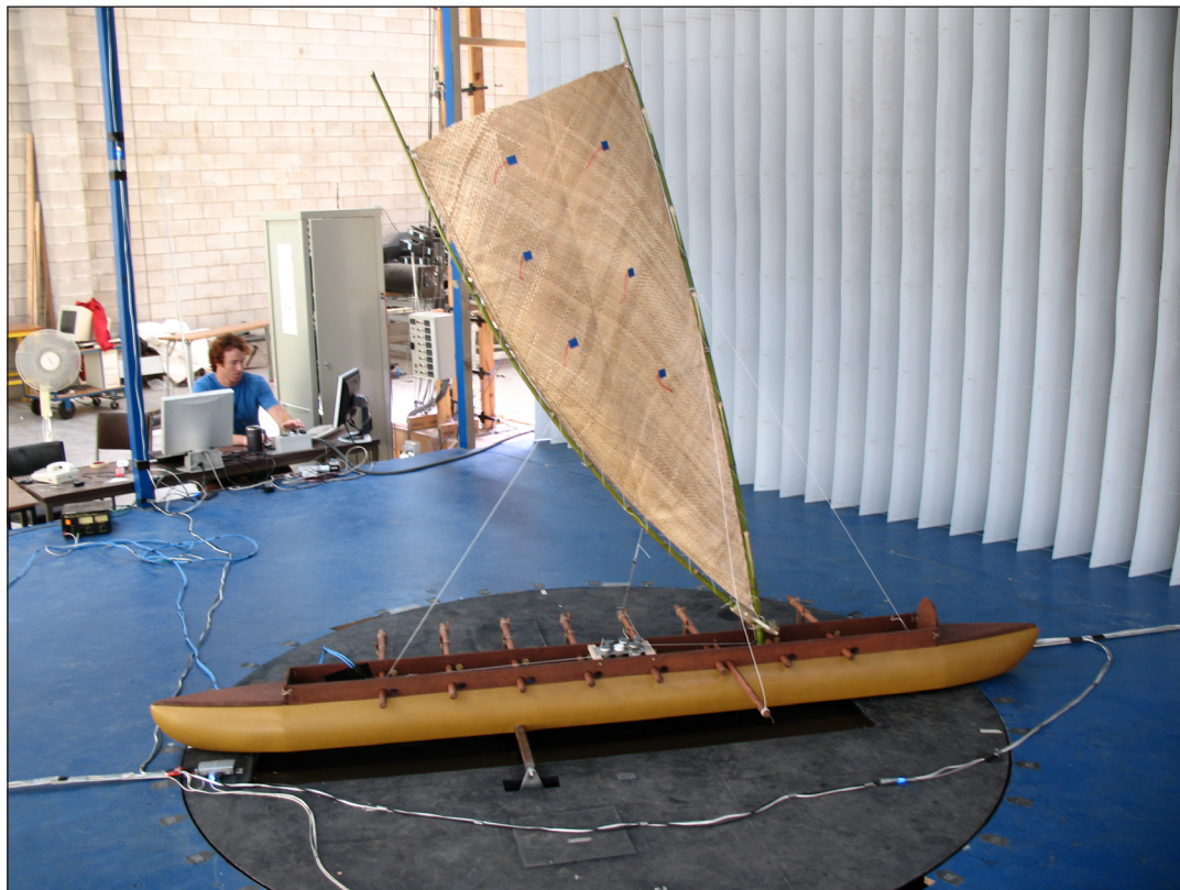
Figure 7. An Oceanic spritsail of a generalised East Polynesian form was tested at the Yacht Research Unit at the University of Auckland. It was mounted on a balance embedded in a turntable in the Twisted Flow Wind Tunnel. The model was tested at angles to the wind between 30^\circ and 180^\circ , at 10^\circ intervals. The trim was adjusted by small electric winches on the model using tell-tails on the sail to get the trim resulting in the largest driving force. The sail was made of finely-woven pandanus and the spars were bamboo.
