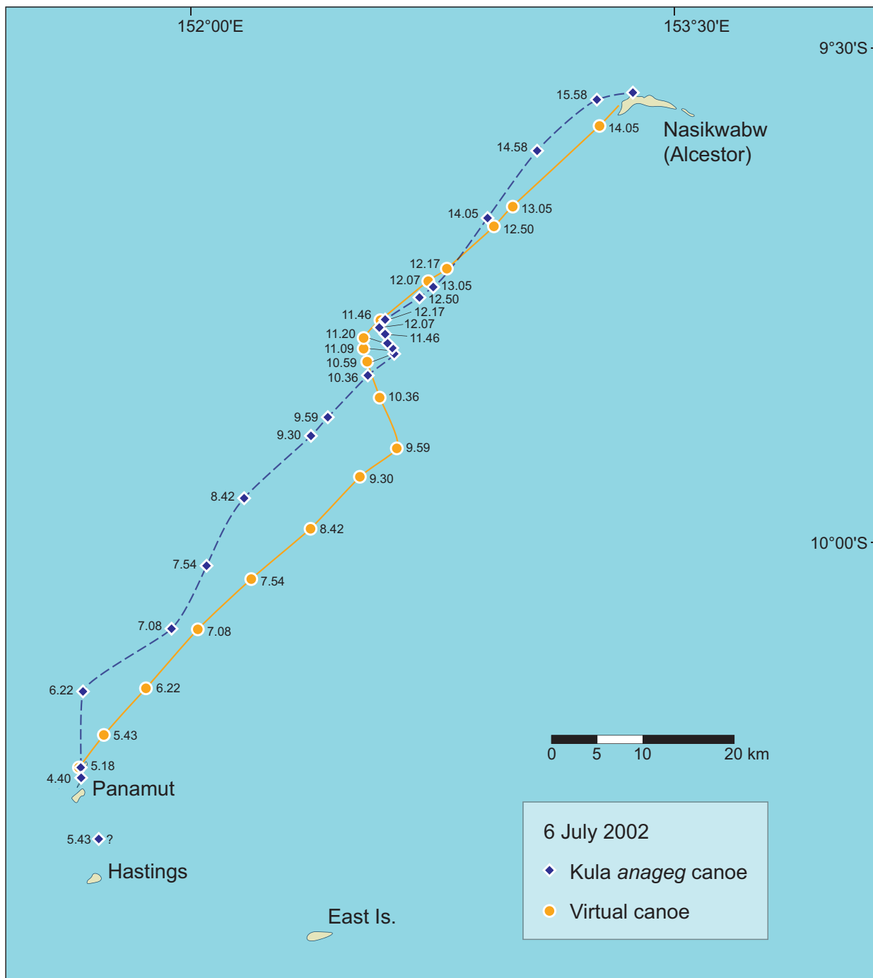
Figure 13. Leg 2 was a distance of 96 km. The wind direction shifted from 170° to 190° during the day (180° is from due south), and the average wind speed increased from 19 to 22 knots (35 to 41 km/hour). There were gusts and squalls. The virtual canoe travelled around 54 sea miles at an average speed of approximately 5.6 knots (10.4 km/hr) at a true wind angle (TWA) of around 135°. The nagega sailed nearly directly downwind in the early morning and at around 160° TWA between 7.00 and 9.00 am. It experienced some dangerous mishaps during the voyage.
