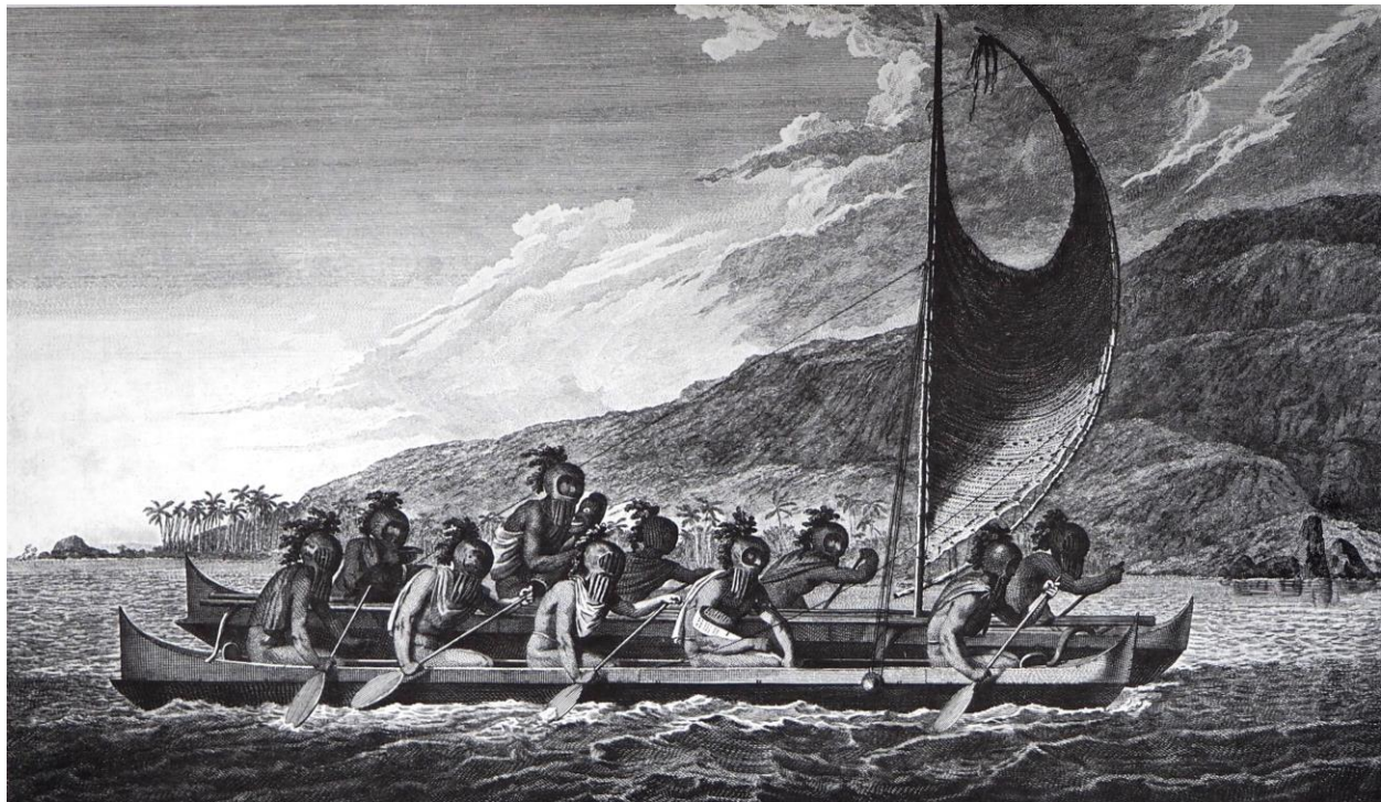
Figure 6: A Hawaiian canoe with a masked crew. Engraving after Webber by Grignion. The line lifting the boom and pulling the tops of the spars together creates the illusion of a crab-claw shape. This line was used for depowering (reefing) the top of the sail by forming a funnel from which air could escape.
