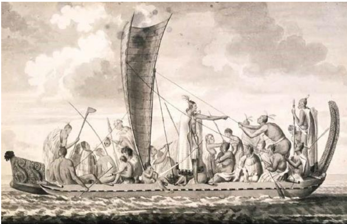
Figure 4. A drawing of a double canoe by Sydney Parkinson, 1770, British Library, London: Add.Ms.23920 f.49. Here the starboard spar has more support from lines attached about two-thirds of the way up. However, the port (adjustable) spar is forward of the starboard spar for this point of sail.
