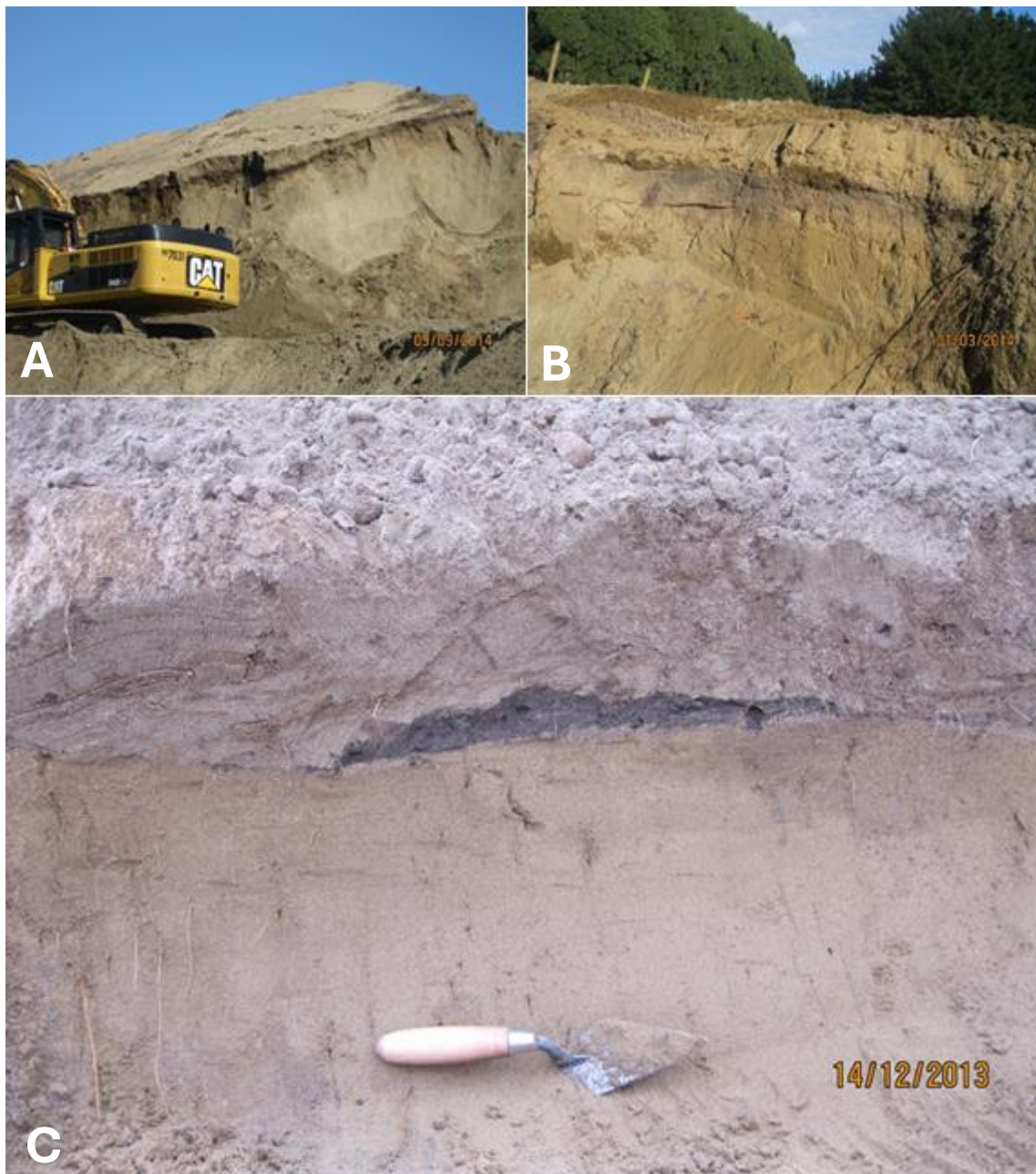
Figure 24: Examples of buried topsoils or dune horizons. A: shallow buried topsoil between dune deposition episodes, revealed by machine cutting. B: shallow buried topsoil between dune deposition episodes, revealed by machine cutting. C: buried topsoil between dune deposition episodes, showing difference in sand colour and consolidation.
